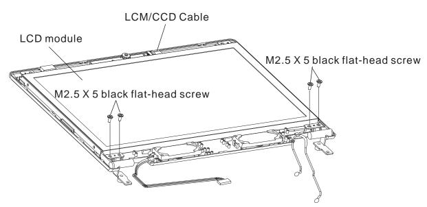
Figure 4-19 Removing the LCD module and screws
